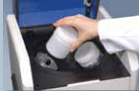
The containers are set in the mixer.
